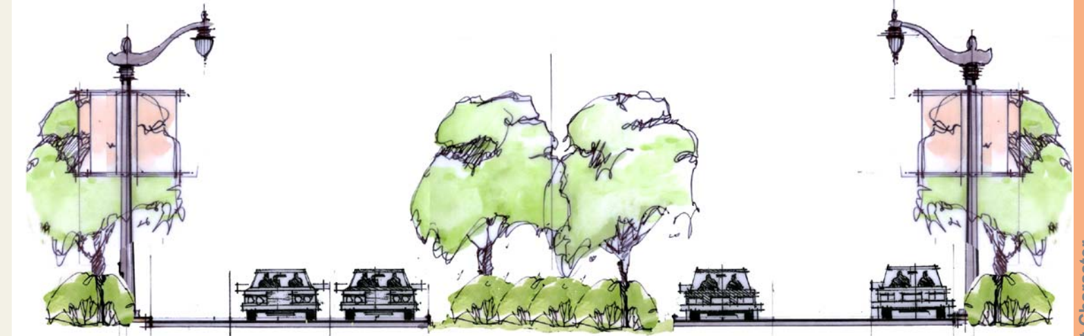
Proposed section through S.R. 249 showing landscape medians, street lighting and landscaping of edges
